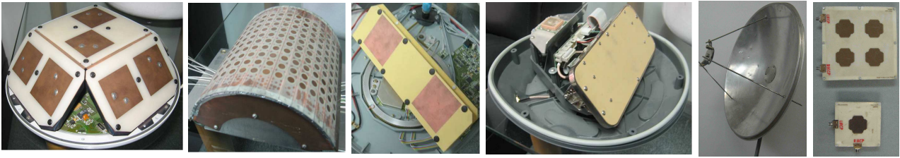
Fig. 2. Variants of steerable, switchable or fixed antennas for the Earth station and for the satellite station
