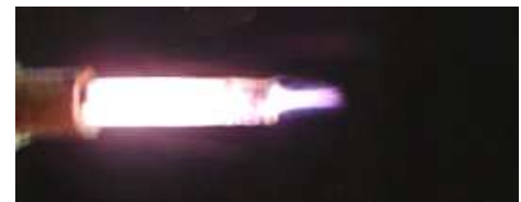
Fig. 7 Ar-plasma jet in atmospheric pressure, experimentally observed in Faculty of Physics
