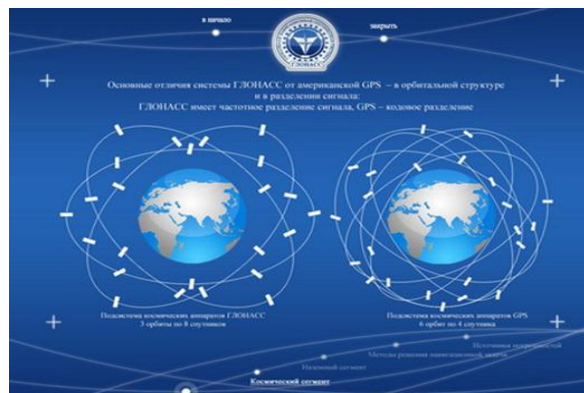
Picture 3. GNSS configuration GLONASS (left) and GPS (right).
